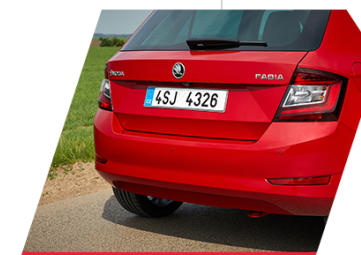
New rear: tail lights and new bumper with integrated reflectors
