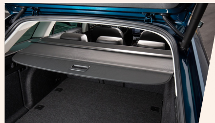
Automatic retractable load cover
