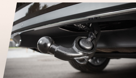
Retractable tow bar with an adapter
