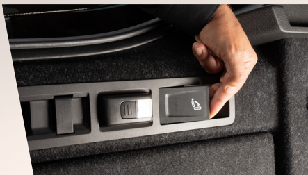
Button-operated folding of rear backrest from the boot
