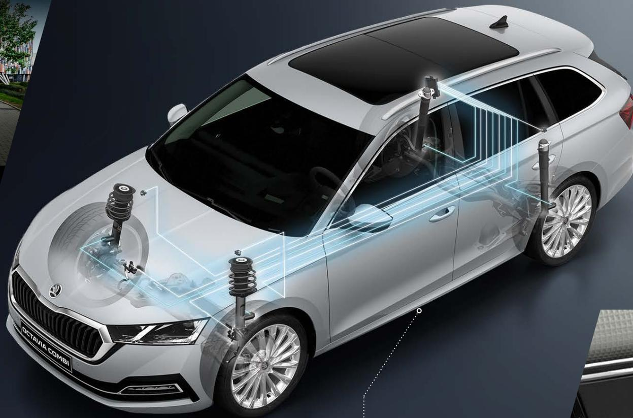
Adjusted using Driving Mode Select via the MODE button; settings are displayed on the infotainment system
