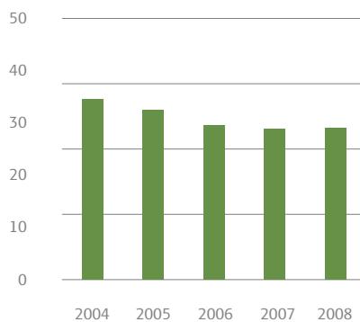
Volatile Organic Compounds (VOC) Emissions per m 2 of Vehicle Body Surface Area Painted
