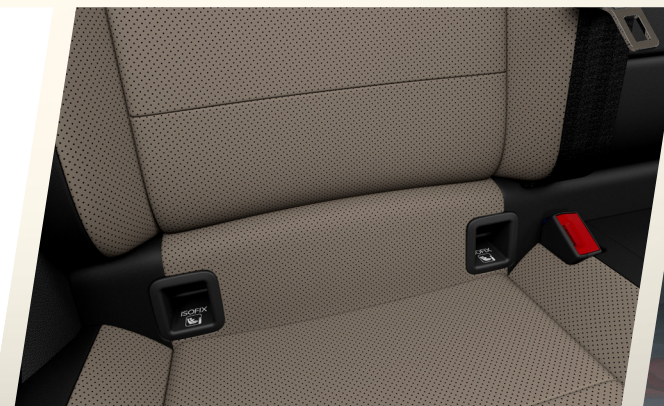
Isofix anchors & top tether anchor points
