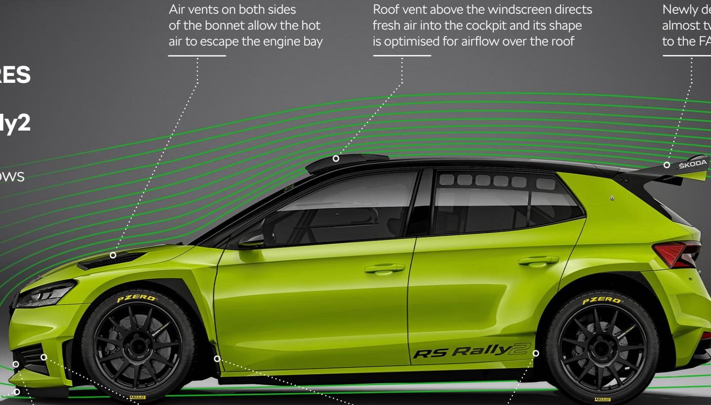
Air vents on both sides of the bonnet allow the hot air to escape the engine bay
