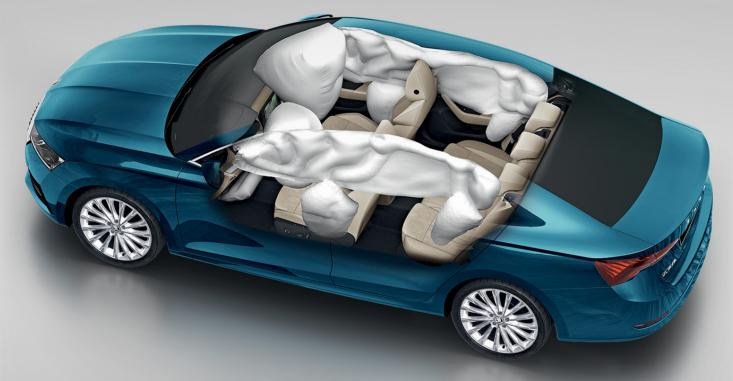
In addition to driver and front passenger airbags, front side airbags and curtain airbags come as standard, while rear side airbags are available as an option for all ŠKODA models. Except the ENYAQ iV series, knee airbags can be fitted in every ŠKODA model.
