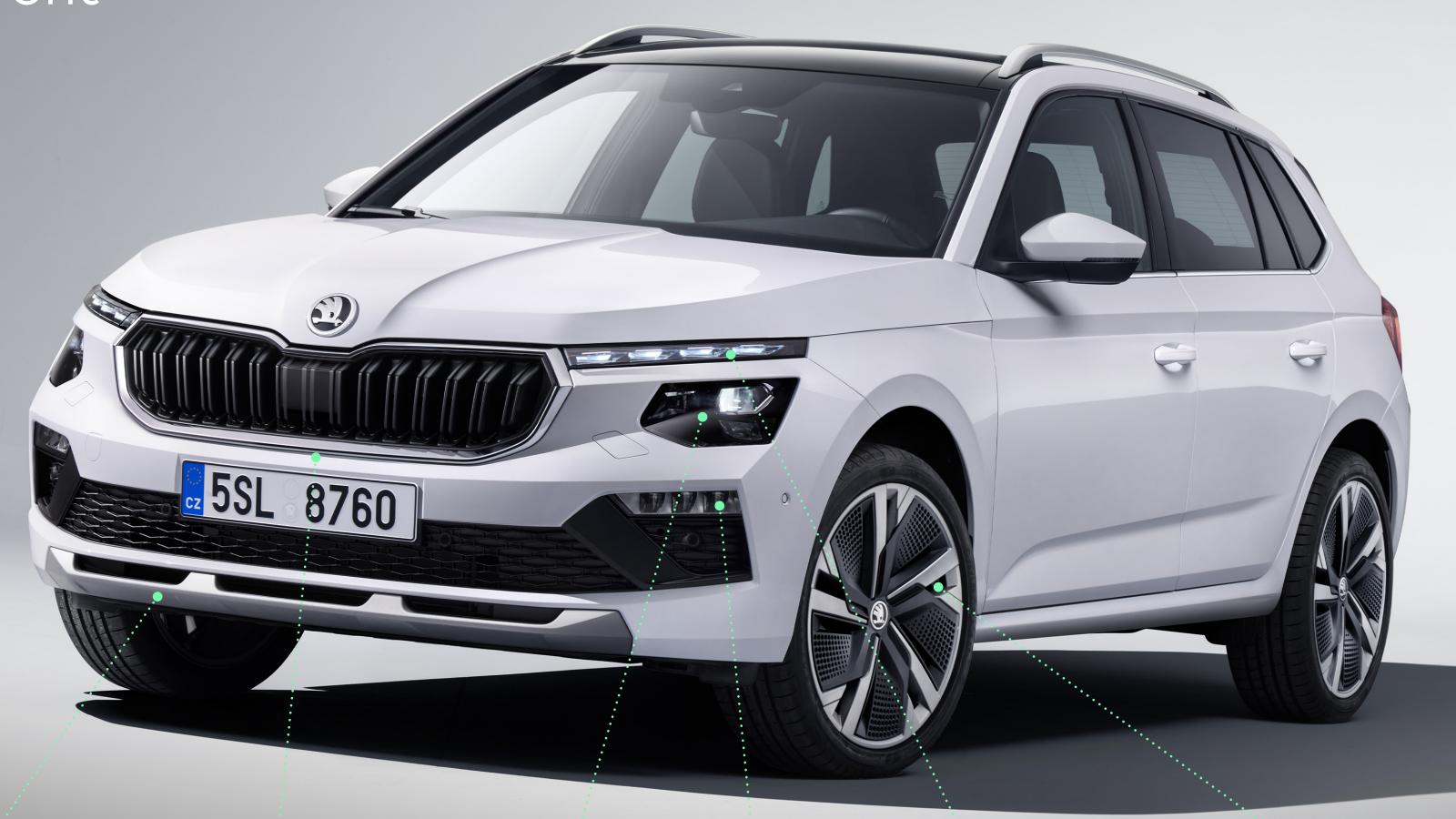
Robust silver diffuser with three openings for typical SUV underbody protection Larger and more upright grille TOP LED Matrix headlights LED front fog lights
