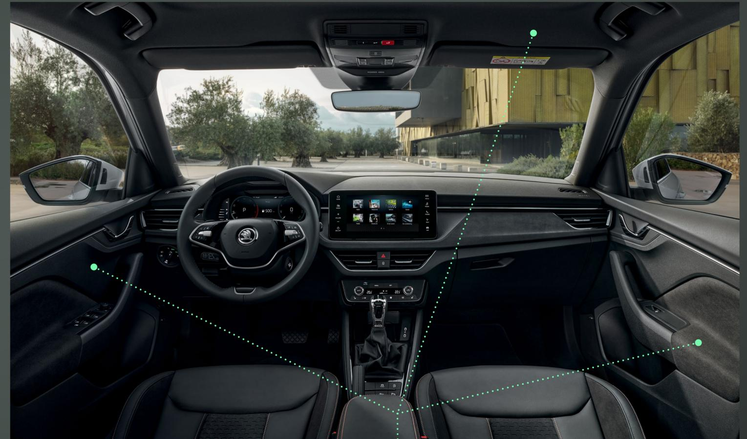
Wood flour, recycled materials, hemp and kenaf are used in the door panels and headliner
