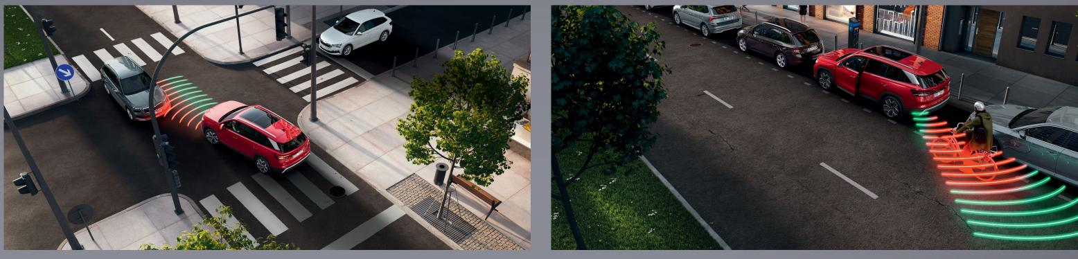
Turn Assist and Crossroad Assist Enhanced safety with Turn Assist and Crossroad Assist: Proactively monitoring junctions and oncoming traffic, these systems alert and autonomously brake to prevent collisions during turns and at obstructed views, ensuring safe manoeuvres at speeds up to 30 km/h.
